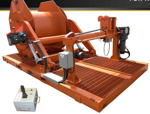
IMG Cable Repair Reeler consists of a Stationary Reel, Lifter Reel and Worktable. Lifter Reel allows for loading and off-loading from site loader attachments. Units can be supplied with all required testing and cable vulcanizing equipment.
